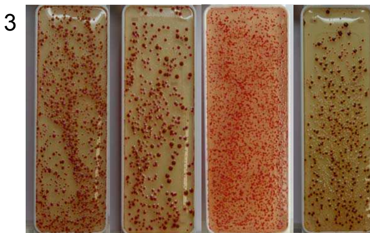
Bottom left: Obernkirchener Sandstone OK A2 NF2 demineralized water, disinfected with ultrasonic equipment A3) water from the storage vessel B3) outflow 0,025 ml/min (15.8.2013) C3) inflow behind the pump (pump purge setting 5 ml/min)(28.8.2013) D3) outflow 0,5 ml/min (20.8.2013) also colorless dots are bacterial colonies
