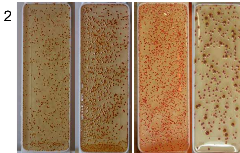
Center: Obernkirchener Sandstone OK A14-A demineralized and boiled water A2) sampling water from the storage vessel B2) outflow, short after iso-Propanol was used, 0,05 ml/min C2) outflow D2) outflow after weekend with 0,025 ml/min (15.7.2013)
